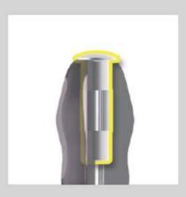
Ergonomic handle with built - in Go - thru mechanism absorbs fierce impact. Blade embedded tightly in into handle that the impact can be conveyed to tip. One-way thread on rivet reduces the vibration during impact.
